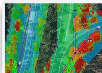
Hazard mapping on an orthophoto
