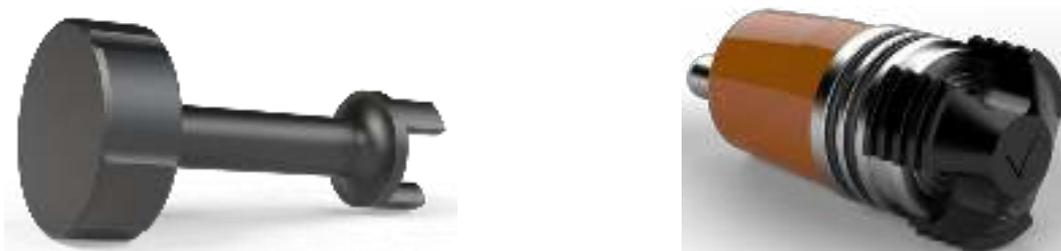
The three prongs should be carefully inserted into the black screw cap of the Pressure Module and turned counter-clockwise (when looking directly at the module) to loosen it. Keep turning until the Pressure Module gently pops out of the socket. The tool will engage with the Pressure Module and allow you to very gentle pull if required.
