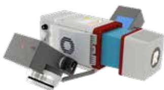
with two Sony Alpha 6000 cameras (oblique mount)
