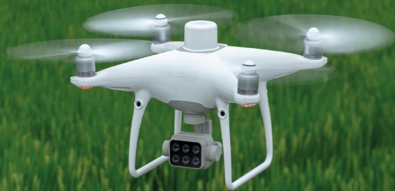
Gather precise plant-level data using the P4 Multispectral – a high-precision drone with a seamlessly integrated multispectral imaging system built for agriculture missions, environmental monitoring, and more.
