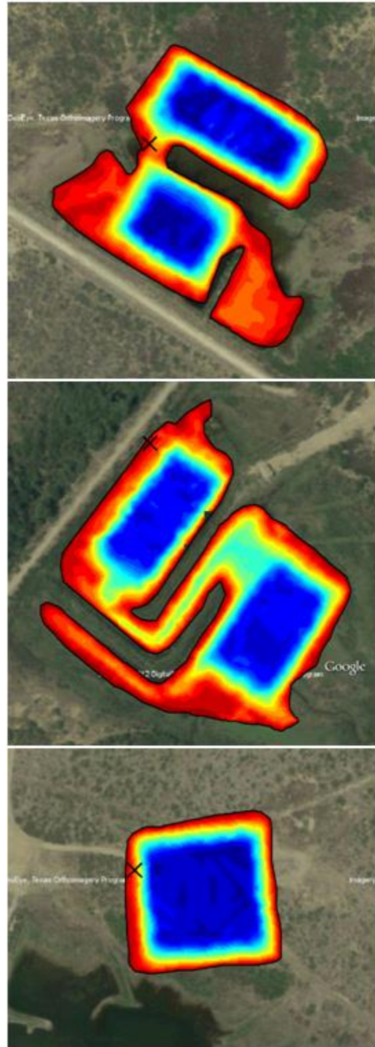
Figure 1. Holding pond bathymetric images, allowing accurate and instant calculation of the water volumes.
