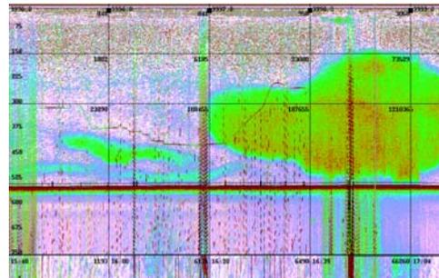
Figure: Echogram of herring concentration in Ofotfjorden and NUI Explorer swimming through the shoal. Surveyed by the Institute of Marine Research Institute, Bergen, Norway and NUI AS.
