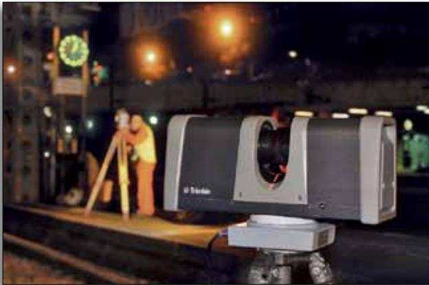
angles and poor lighting conditions might affect the precision of measurements to the tracks. To ensure that these difficult measurements met required precision, the technicians used the 2-pass configuration of their Trimble FX Scanners.
