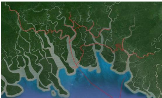
All of the rivers were uncharted before the ship traveled upstream. With incomplete tide station coverage, determining the ship's path was a complex calculation. Despite this, and complicated by a bore tide, YWAM were able to take their vessel 75 km upstream in the Bamu River, Western Province with no published charts. However the most startling example of the benefit of the YWAM hydrographic survey approach took place in the second year of operation. Jeremy described the events:
