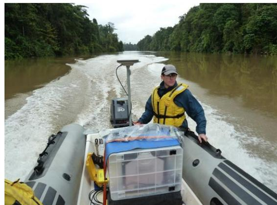
The CEESCOPE was an ideal choice for the YWAM surveys; the one-box survey system was easy to swap between the two available 4.2m and 5.2m boats. It could be used without an acquisition PC on the survey launch if needed - all data recorded on the internal memory, and could run on its own battery power for an
