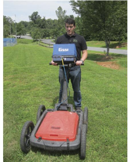
*Mitch Ross at ISS uses ground-penetrating radar to locate utilities.*
