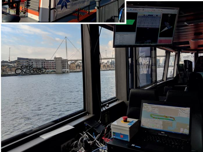
» Image aboard the Patriot, showing Teledyne PDS controlling the sonar in the top screen, and CARIS Onboard displaying the automatically processed surface on the bottom screen. This demonstrates how the processed data can be used on the vessel to guide the hydrographer without distracting from running the survey equipment.
