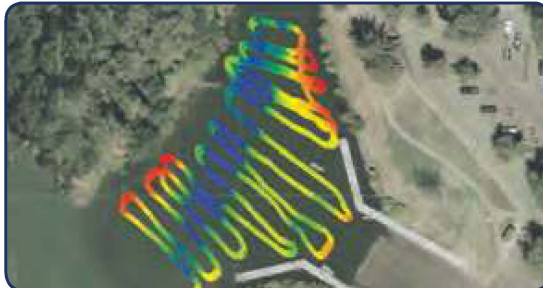
Digital terrain model from single beam echosounder data
