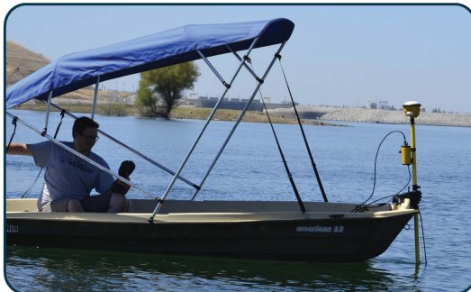
HydroLite-TM Mounted to jon boat bow
