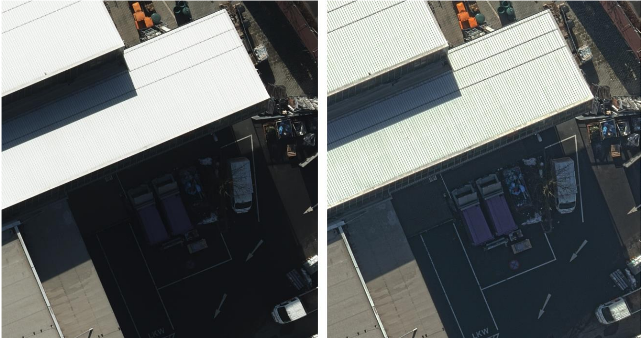
Fig 8: Crop from UltraCam Eagle Prime f210 frame 383: The crop area consists of a high dynamic band width. A high dynamic range (HDR) process was applied to enhance the image and show the details in bright and dark areas.
