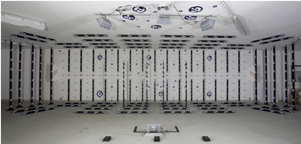
Fig. 1: UltraCam Calibration Laboratory: The three-dimensional calibration rig covers a horizontal field of 12 m.
