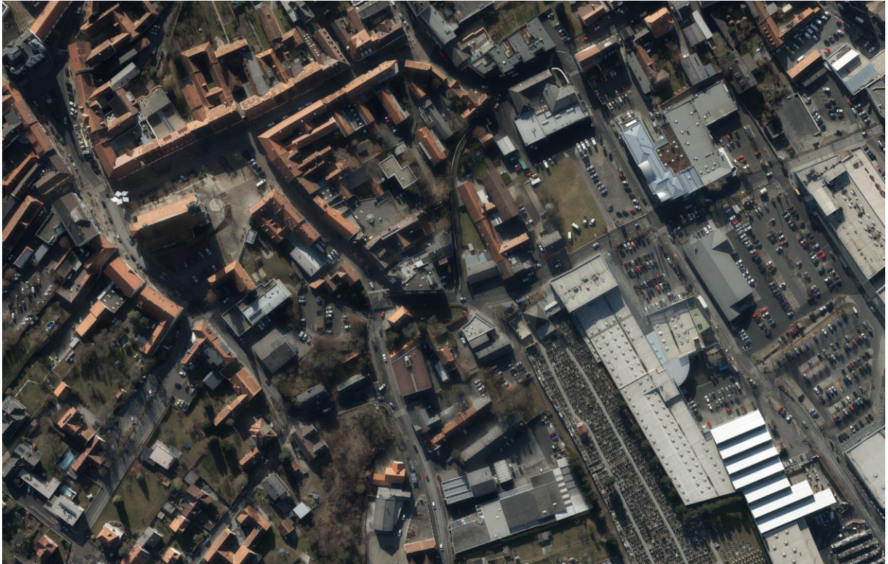
Fig 5: UltraCam Eagle Prime f210 full frame (image 383) with 23,010 by 14,790 pixel. The Image was taken on Jan/12 2016 at an altitude of 1,140 m AGL and 210 mm focal length. The resolution on the ground (GSD) is at 2,5 cm. Long shadows and brownish colors from the winter landscape dominate the image content.
