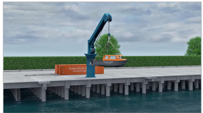
Hoisting eyes are present to deploy the vessel from almost any dock.
